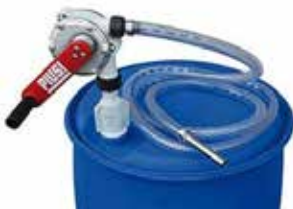
ADBLUE Hand Pump PIUSI DN50 Male BSP Thread, 2.5m delivery hose, stainless steel spout, 38L per 100 revolutions
